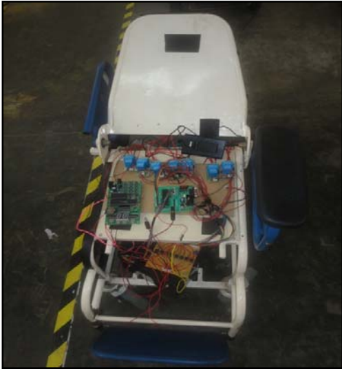
Fig 4 : Speech recognizing powered wheelchair for disabled – electronic components
